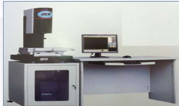
Two dimensional projector: Tileinspection
